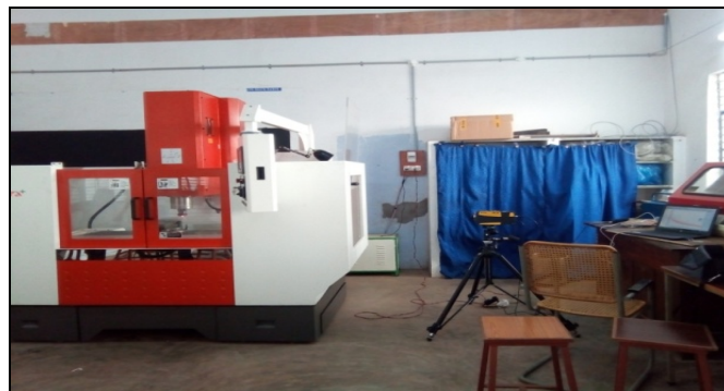
Figure 1: 3-axis CNC vertical milling machine with Laser Doppler Vibrometer (LDV) arrangement
