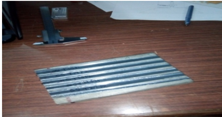
Figure 2: The machined AISI 316 Austenitic Steel work piece
