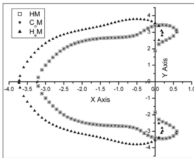
**Figure 1.** Comparison of Stability regions for the fifth order RK based on HM, C<sub>o</sub>M & H<sub>e</sub>M
